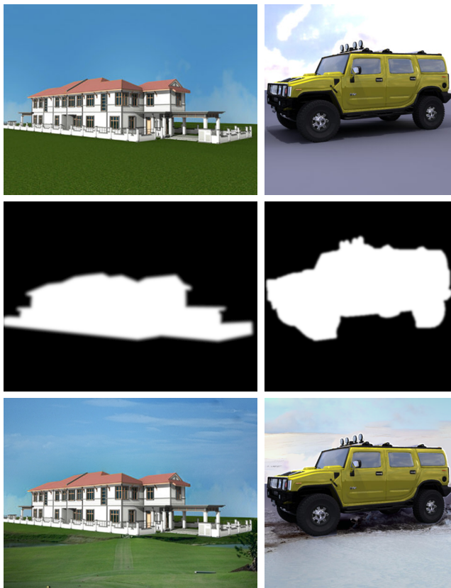
Fig. 8. Realistic backgrounds for CG models. In some cases, a user may not want regions of the image replaced. The user can specify an alpha mask (middle row) and the system will operate outside the mask, thus creating a realistic context for a rendered model (bottom).
